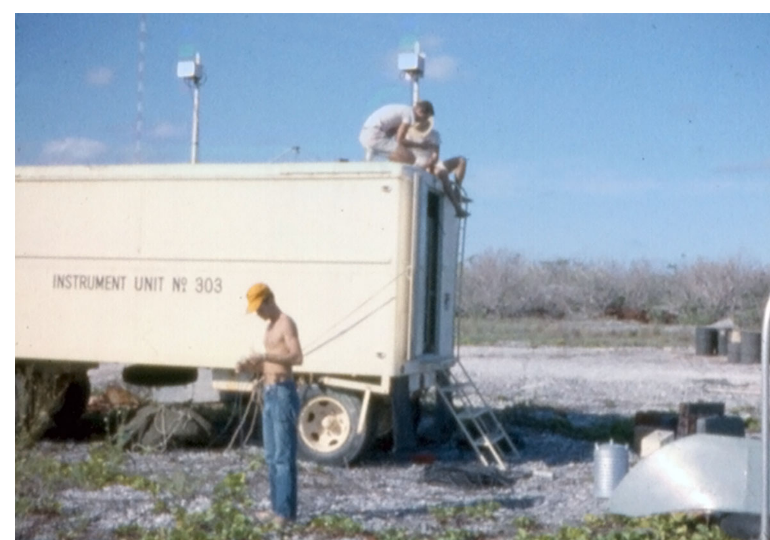
Doppler Shift satellite tracking van with crew members John Ruminer, Ron Streich, and John Walker. The tracking frequency pairs used were 150 & 300 MHz and 200 & 400 MHz
